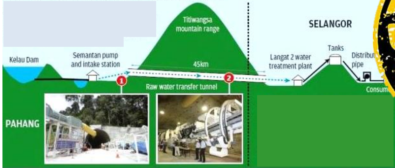
Pahang – Selangor raw water supply scheme
