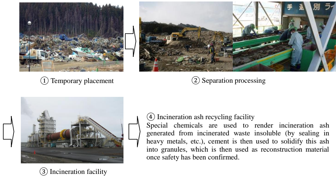
Figure 10: Flow of disaster waste processing
